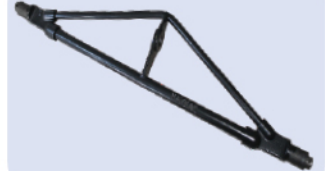
KYK-207-60-M 60 kN MÜSELLES ORTADAN BAĞALI 60 kN BRAKE TRIANGLE MIDDLE CONNECTION
